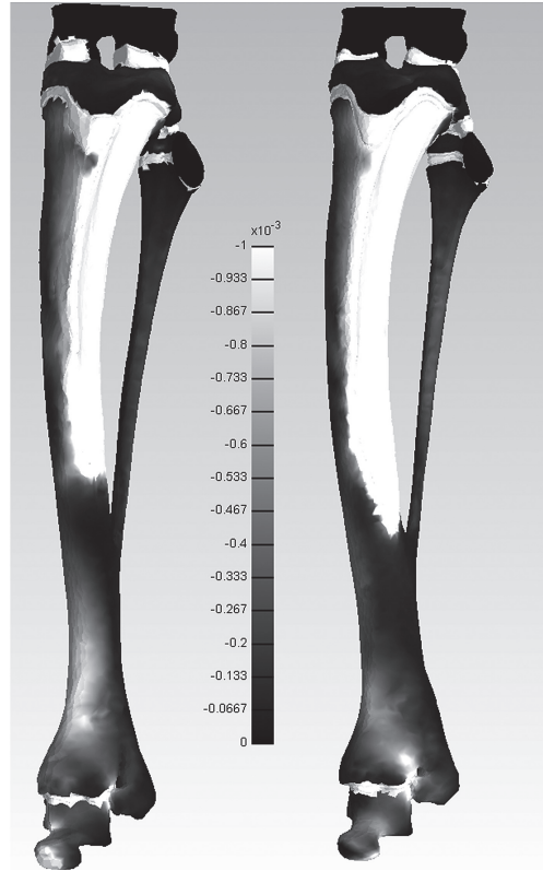
Figure 3. FE models, showing compressive strain across the unstimulated geometry (left) and the stimulated geometry (right) under identical loading conditions. White indicates highest strain, black the lowest.
